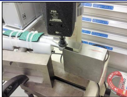
**The moment load at the time of rotation stop is measured by pushing a push-pull gauge onto hand piece head**
